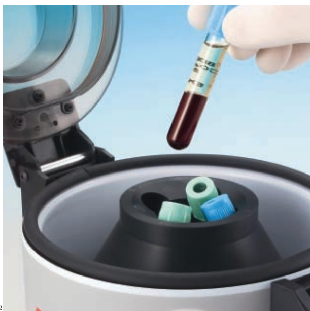
Owing to their aerodynamic construction, fixed-angle rotors can attain much higher speeds.
