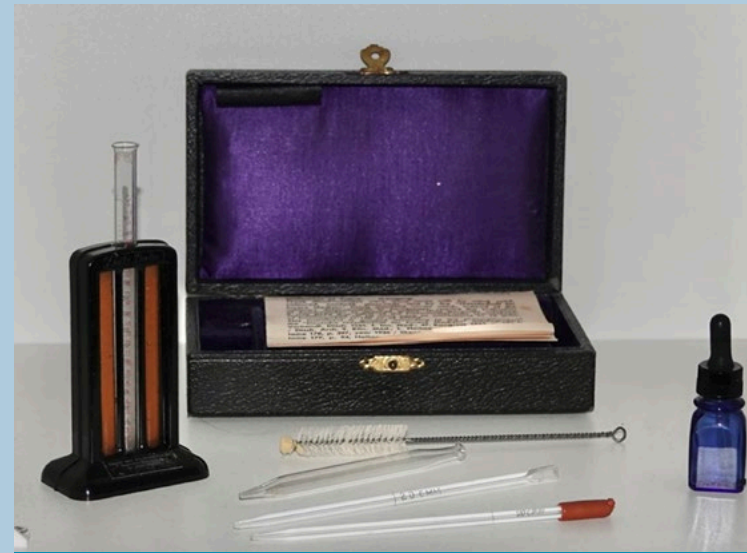
Haemoglobinometer with graduated tube, standard solution, 20 cmm pipettes, N/10 hydrochloric acid and a cleaning brush (IBMS Instrument Collection).
