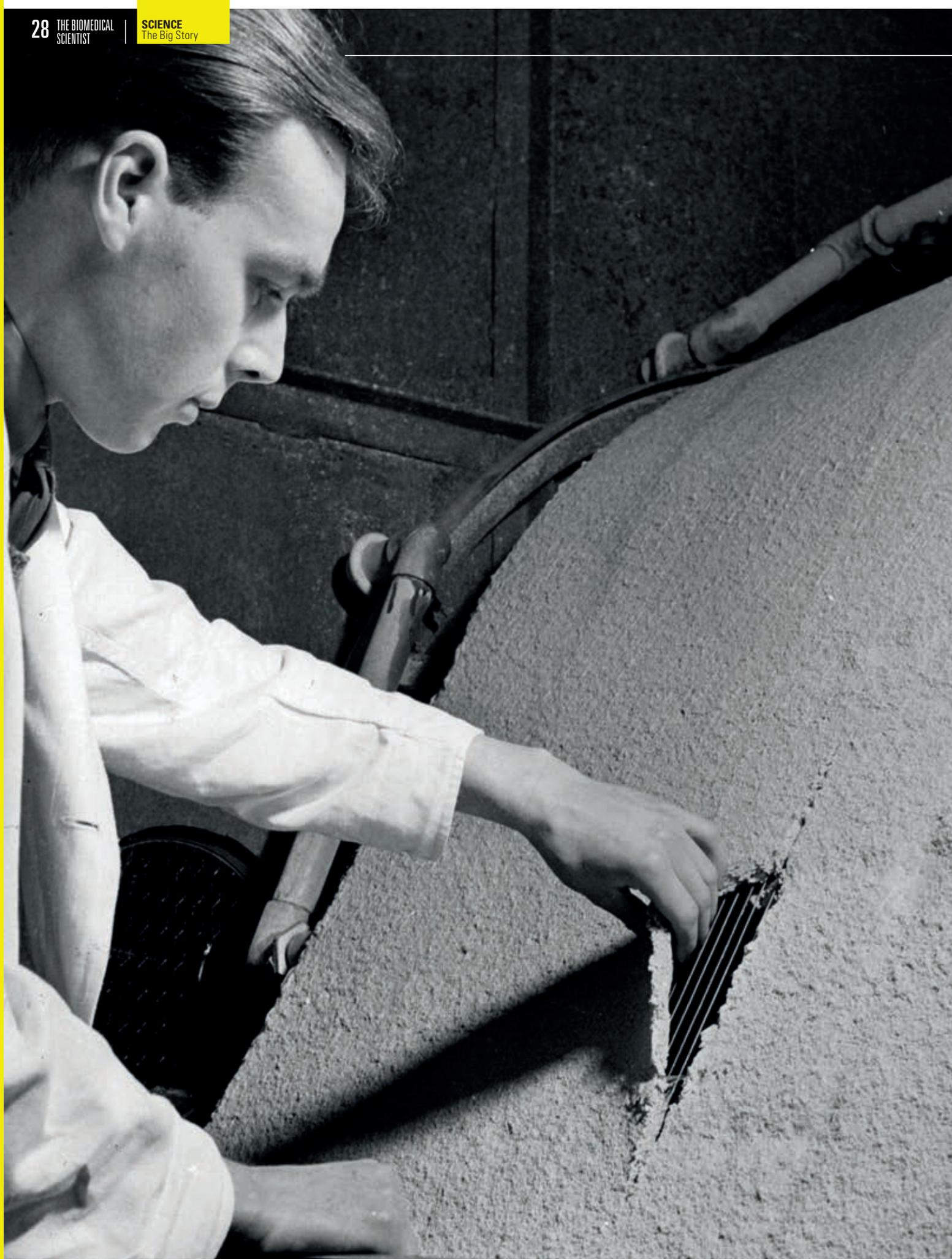
**Below.** A man pulling off the filter during penicillin manufacture at Glaxo, circa 1956.
